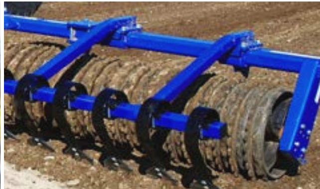
Mounted with hydraulically adjustable cracker board.
