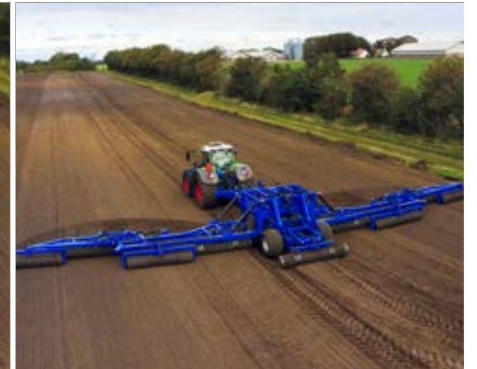
4. When the roller sections are in the working position, the 2 hydraulic weight distribution systems are at the correct working pressure and in the floating position, the wheels are automatically raised free of the ground.
